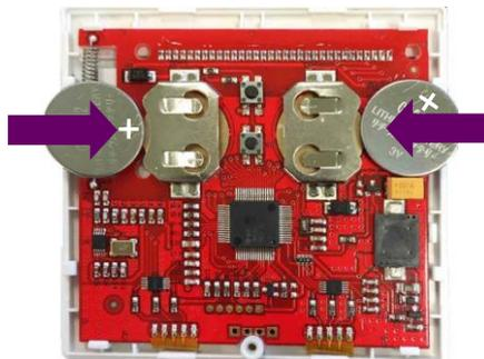
put in the two batteries mind the right polarity
