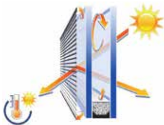
STANDARD SHADE FABRIC 75% of heat is transmitted 25% of heat is reflected
